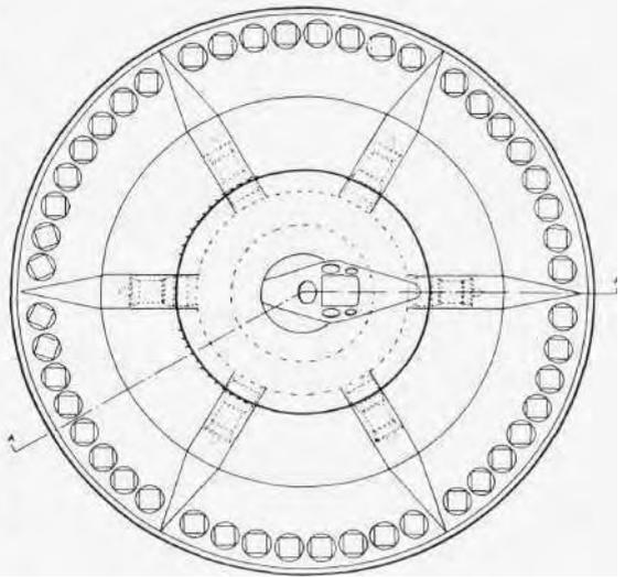
Right: General arrangement of the proposed Avro Project 1794, showing arrangement for its six Viper turbojets.
