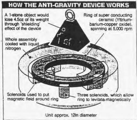
tures. The team was carrying out tests on a rapidly spinning disc of superconducting ceramic suspended in the magnetic field of three electric coils, all enclosed in a low-temperature vessel called a cryostat.
